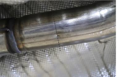
To make it easier to cut the exhaust we recommend removing it from the car. Find the indent just before the resonator to mark out the cutting line. Cut along the line and de-bur the edges. If fitting with the original GPF-back re-fit this now and then fit the Scorpion GPF delete following the line diagram on the first page. If fitting with the Scorpion GPF-back you do not need to use the supplied adaptor.
